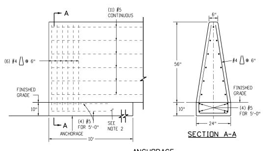
ANCHORAGE BARRIER ELEVATION VIEW INCLUDING REINFORCED ANCHORAGE AT END.
