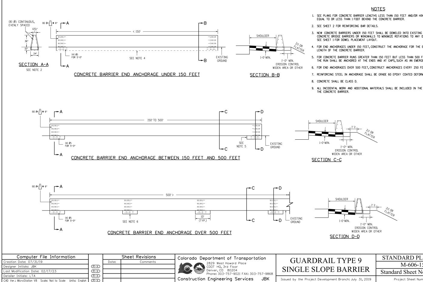
1. SEE PLANS FOR CONCRETE BARRIER LENGTHS LESS THAN 150 FEET AND/OR HINGE WIDTHS
