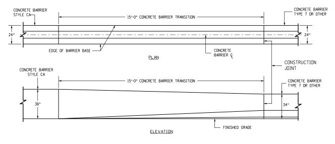
TRANSITION CONCRETE BARRIER TYPE 9 TO CONCRETE BARRIER TYPE 7 OR EXISTING
