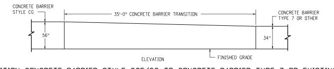
TRANSITION CONCRETE BARRIER STYLE CGE/CG TO CONCRETE BARRIER TYPE 7 OR EXISTING
